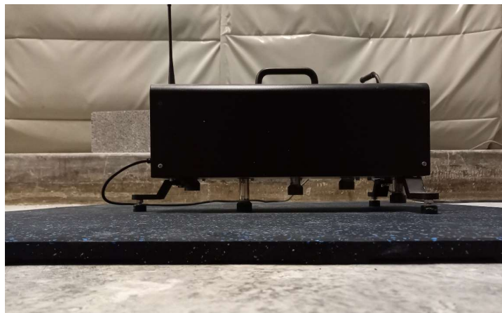
photo: detail with the tapping machine on one rubber tile
